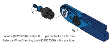
Arrange the contacts according to the color coding as on the table shown below into the contact carrier (5) (Ethernet-standard).
