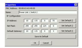
Figure 2: HiDiscovery – IP parameter assignment
