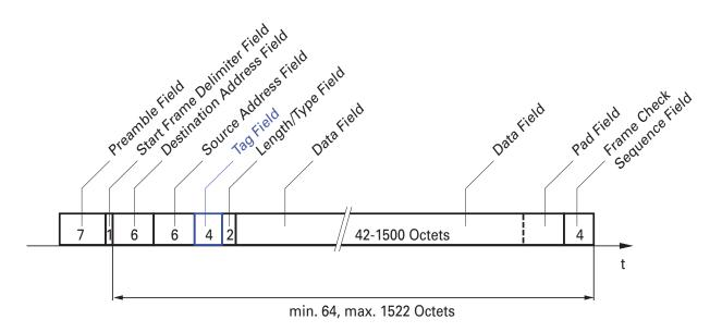
Figure 16: Ethernet data packet with tag
