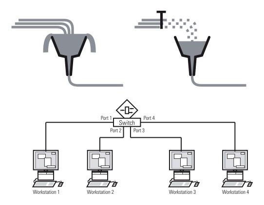
Figure 18: Example of flow control
