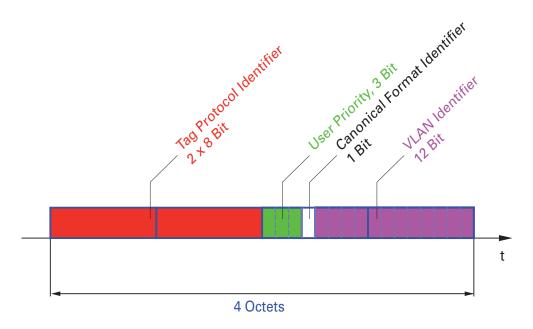
Figure 17: Structure of the VLAN tagging
